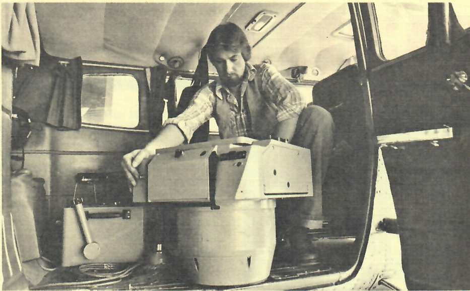
Sidwell photographer mounts 12" focal length camera in airplane TWELVE INCH CAMERA INCREASES MAP ACCURACY
